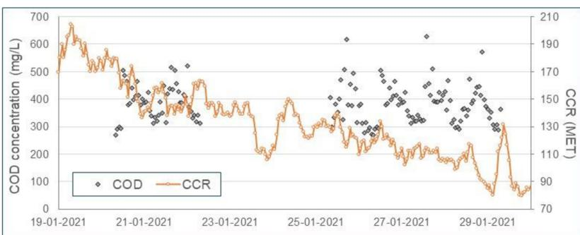
Figure 2 – Time-series of SENTRY sensor data (CCR) and COD measurements for a 10-d period.
