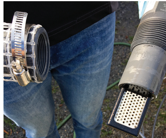
Protective screen meshes are available for sensors installed in high-strength waste streams.
