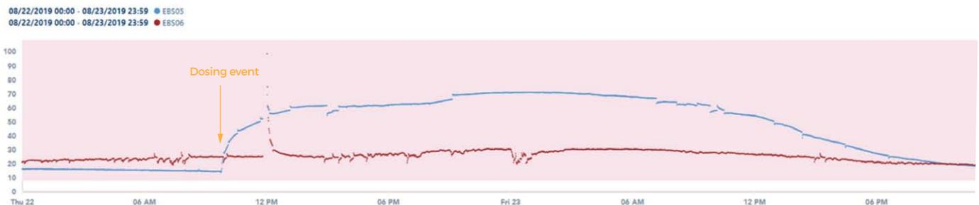
Figure 4: Dashboard view of MET response to black liquor. The black liquor 385% increase in MET and lasted 27 hours.
